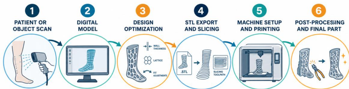
Figure 3. Generic digital workflow for additive manufacturing of prosthetic and orthotic devices, beginning with patient or object scanning and proceeding through digital modelling, design optimization, STL export and slicing, machine setup and printing, post-processing, and completion of the final device.
