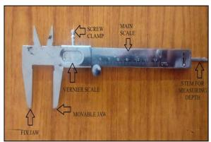
Fig-1: Sliding Verneir caliper
