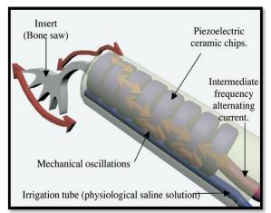
Fig 1: A piezosurgery hand piece with a piezoelectric ceramic chip.<sup>6</sup>
