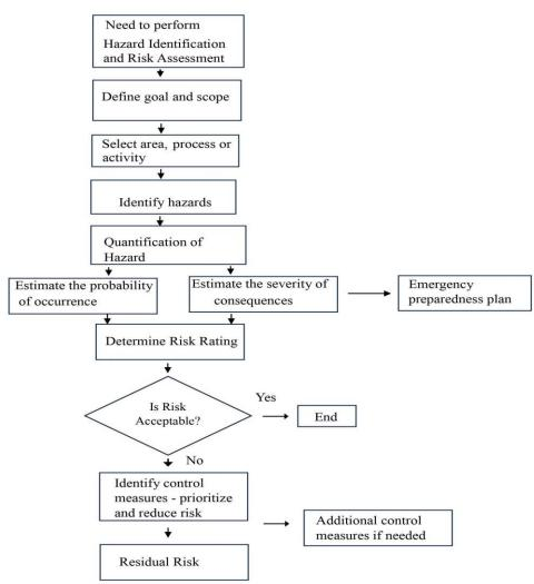
(Figure 1: Flow diagram of Hazard Identification and Risk Assessment)
